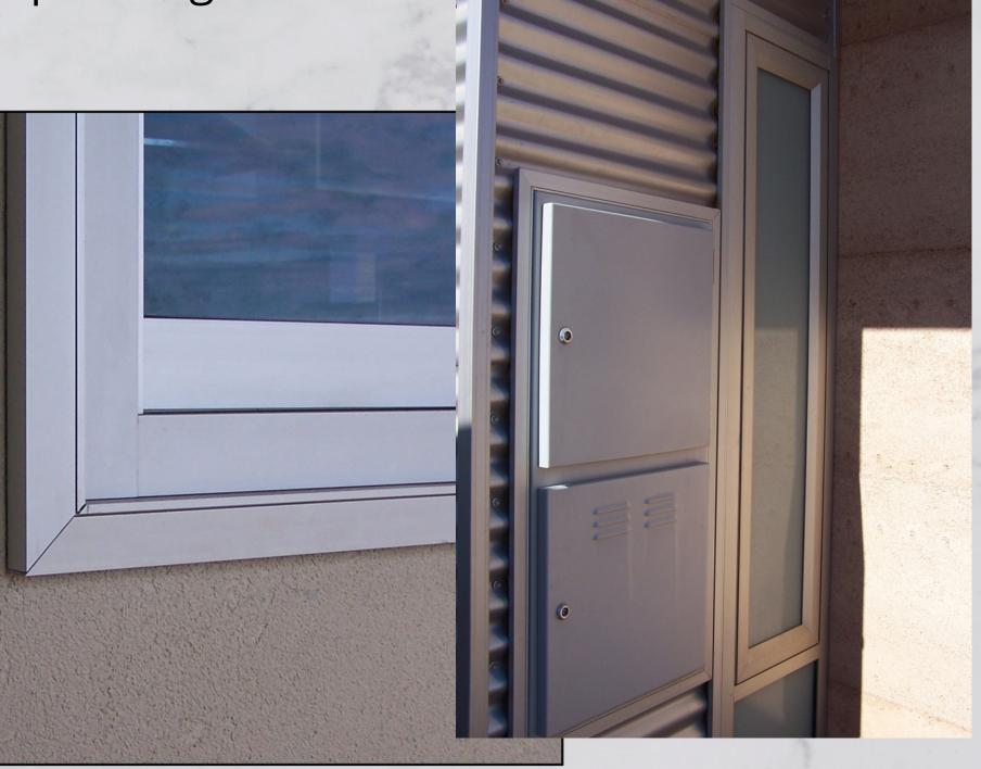
GAS148 - L Frame - Used in all applications to provide a fin and weatherproofing of Window and Door Frames, meterboxes, timber door frames. Mitre cut to provide a continuous fin completely around the frame. Installed in the factory prior to delivery of Windows unless used in a retrofit situation. Can be fitted to existing frames fin or fixed in alternate position.
